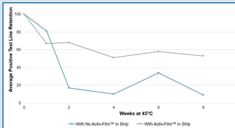
Figure 4: Strep Test Device Stability (With Integrated Activ-Film™ Technology vs. Control)
