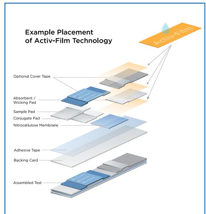
Figure 2: Concept Rendering of Potential Activ-Film™ Integrations for Dipstick or Cassette
